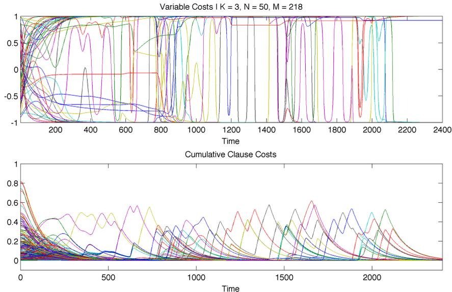
**Figure 4.11** – Solving a 50 variable hard SAT problem with a modified version of the third approach. The system successfully converges to a solution, at the expense of large fluctuation in both variable and cumulative clause weight values
