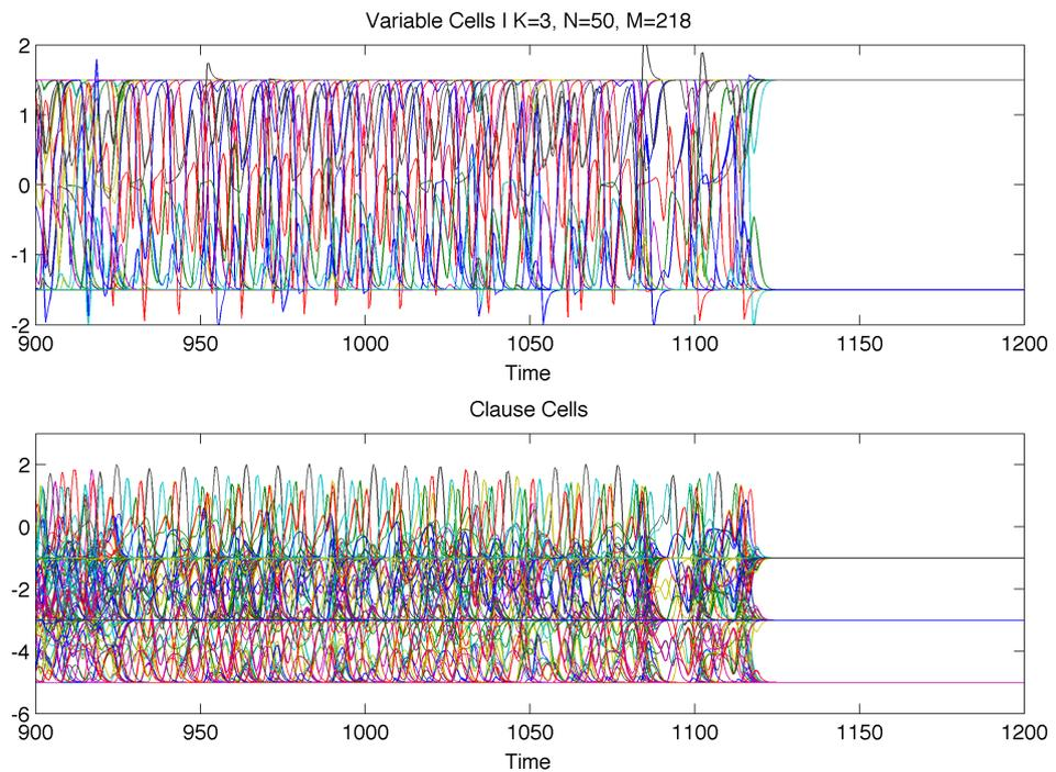
**Figure 4.5** – Using the bounded SAT dynamical system as presented in [MTER12] to solve a problem. A successful solution is found after a long chaotic transient.
