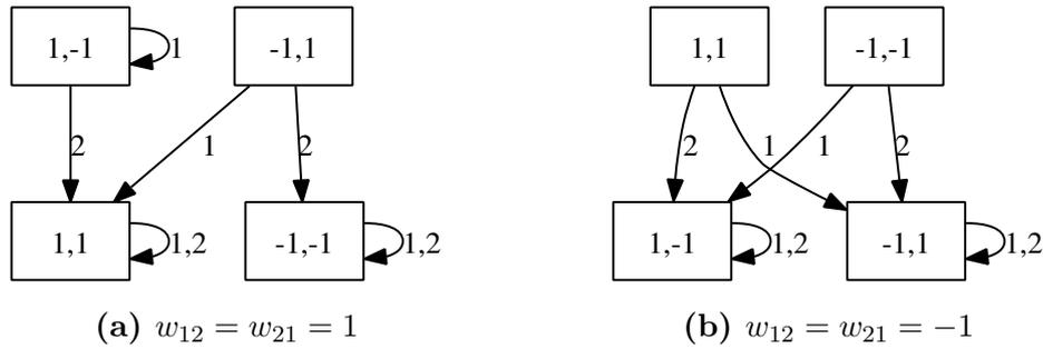
**Figure 2.4** – Orbit plots for the two separate cases. The fixed points in Figure 2.4a are  $[1, 1]$  and  $[-1, -1]$ , and in Figure 2.4b, they are  $[-1, 1]$ , and  $[1, -1]$ . The edge labels represent whether we chose to asynchronously update neuron 1 or 2.
