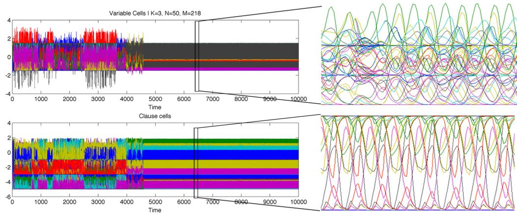
**Figure 4.6** – Using the bounded SAT dynamical system as presented in [MTER12] to solve a problem. The system gets trapped in a limit cycle
