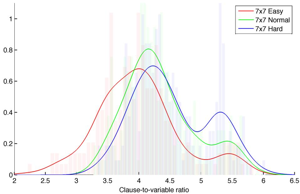
**Figure 5.10** – Probability density functions for  $\alpha$  ratio for “Easy”, “Normal”, and “Hard” problems on a  $7 \times 7$  board. Easy problems tend to have a lower  $\alpha$ . The expected value for “Normal” difficulty is just around 4.3, the hardest region for SAT, while for “Hard” problems, the extra additional constraints shift the expected  $\alpha$  value to the right, making the problem easier again.
