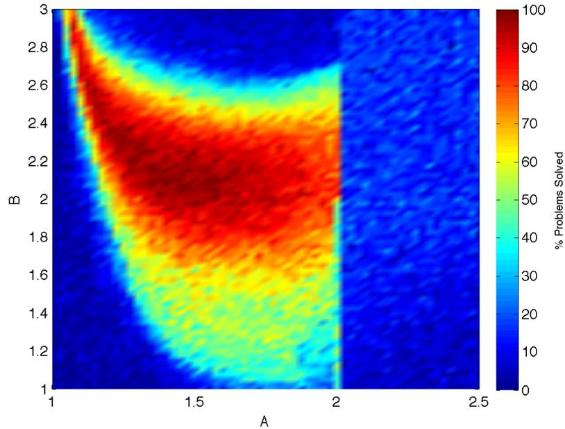
**Figure 4.4** – Proportion of solved hard random 3-SAT problems with time limit 10000 with various parameters of  $A, B$  when solving using the bounded dynamical system for SAT as presented in [MTER12]
