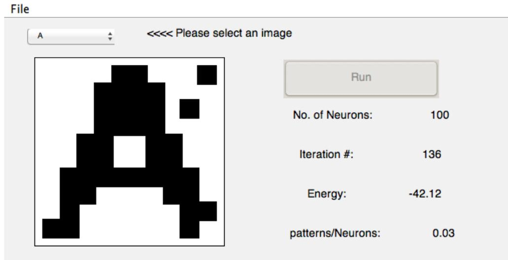
**Figure 3.4** – A GUI showing the application of Hopfield networks to the problem of retrieving a stored pattern. In this case, the stored patterns are binary images of letters, and the task is to reconstruct the original image given a broken image.
